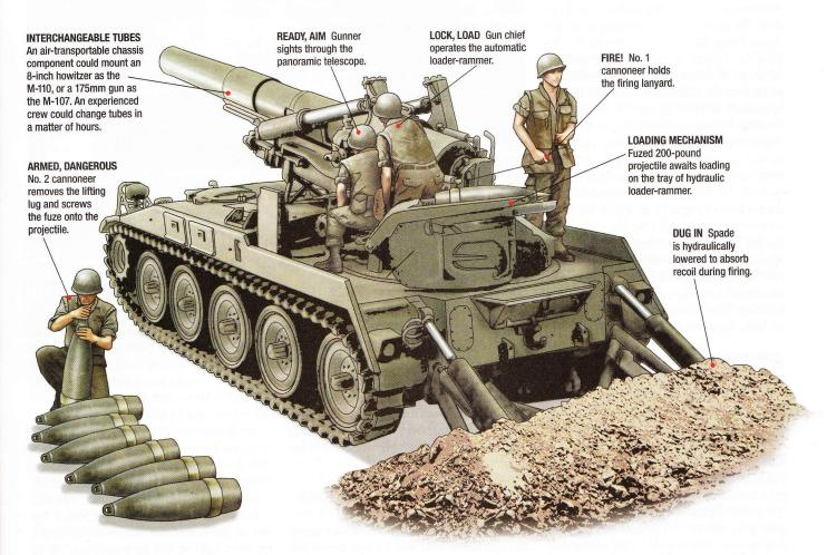
THE SELF-PROPELLED M-110 8-inch howitzer was a corps and division-level weapon that could bust bunkers, destroy enemy infantry in the open and excel at counter-battery fire. Consisting of an M2A1E1 8-inch howitzer mounted on a tracked chassis, the M-110 had a five-man crew in the main vehicle, which carried only two rounds. The other eight crewmen and basic ammunition load traveled in an accompanying M-548 tracked vehicle.
